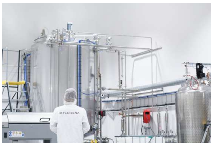
Figure 16: Fungi being fermented in the large vat in a factory producing mycoprotein for Mycorena, a biotechnology company based in Sweden; Image source: New Food
